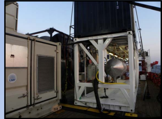
Standard footprint container and frames Mounted and fixed with twist locks Cranes high load capacity
