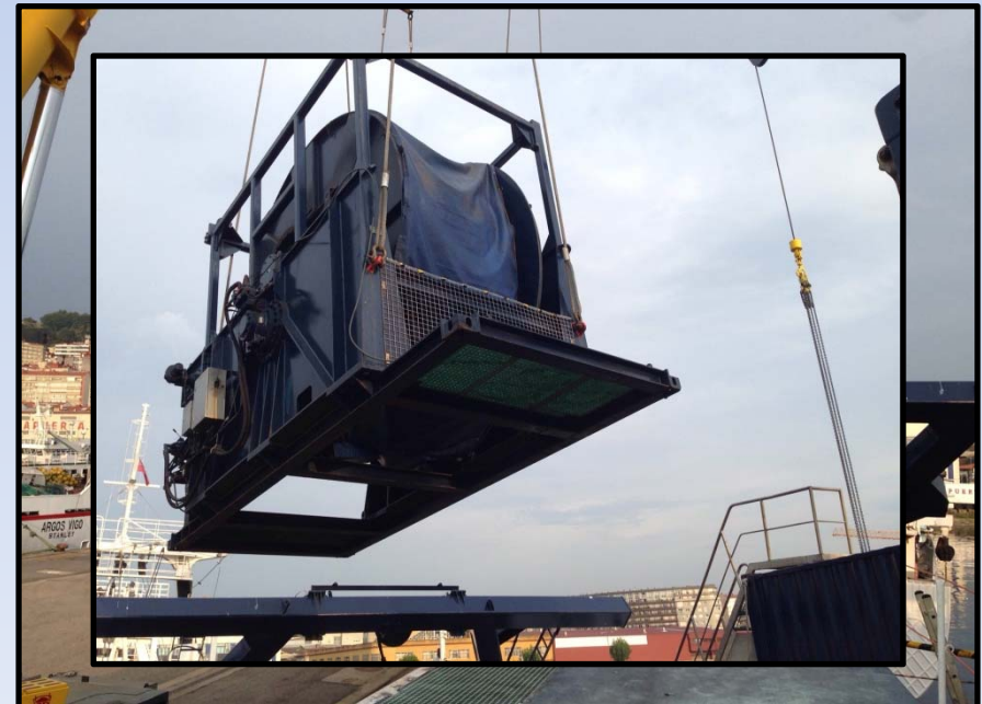
Standard footprint container and frames Mounted and fixed with twist locks Cranes high load capacity
