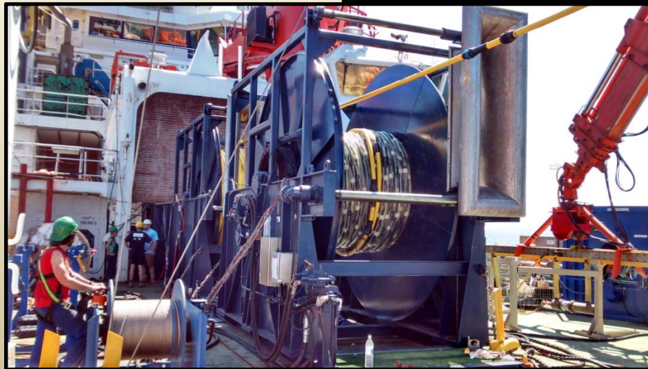
Twin simetric streamer winches
