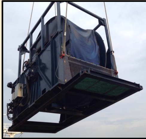
Twin simetric streamer winches
